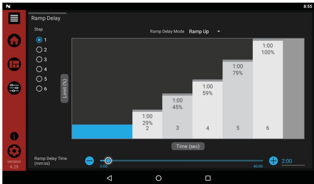
FIGURE 6 RAMP DELAY SCREEN
